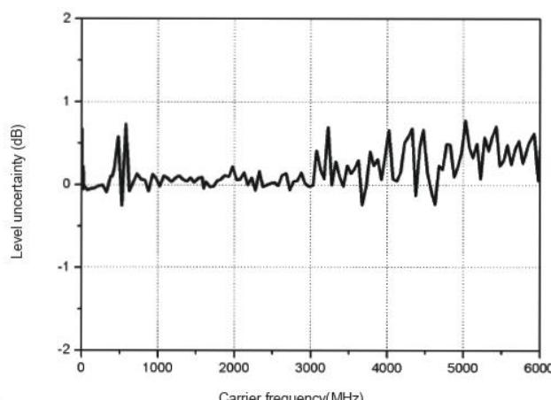
Measured -136dBm output level VS frequency
