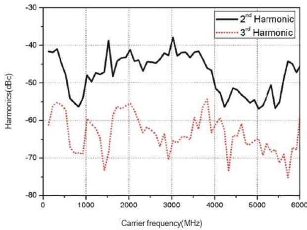
Measured 0dBm output, Harmonics VS frequency
