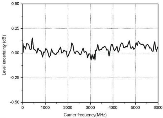
Measured 0dBm output level VS frequency
